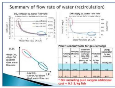
minimal consumption of energy. Energy in RAS systems is mostly used for gas transfer (and combined nitrification in some cases) through the pumping of water and air. As the water head of systems is proportional to the water energy, the idea is to <u>obtain a low head (LH) RAS</u> <u>system</u>, where the water level difference; the head loss due to friction; the velocity head and the pressure head are all minimized.
